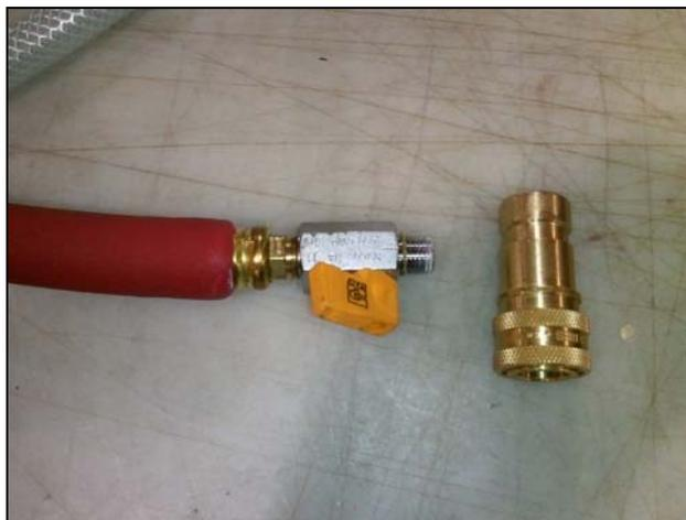
**Drain valve on the bottom of the used tank:**
