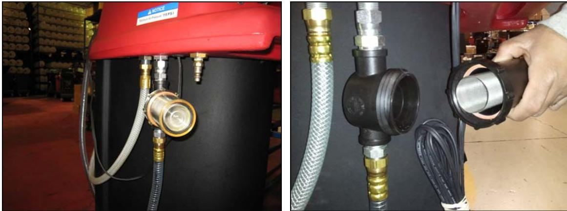
**Some** of the older machines may also have an internal filter that can be cleaned or removed (current production machines do not use an internal filter).
