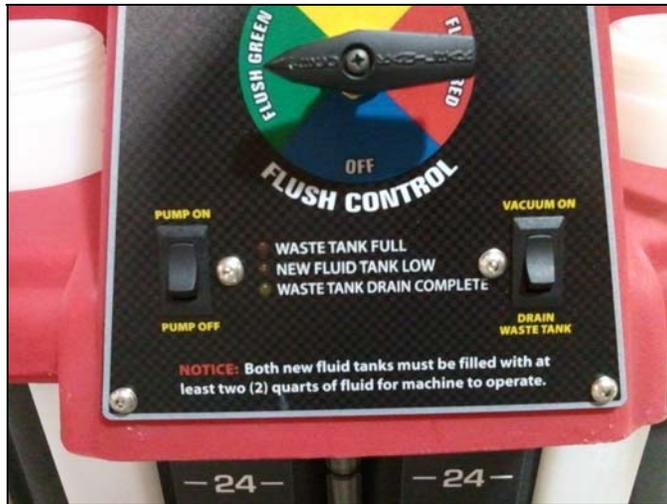
7. New fluid will be pumped through the machine, while the vacuum will pull new fluid through the system into the used tank. If there is any foreign material in the lines, this should force it out after a minute or so.
