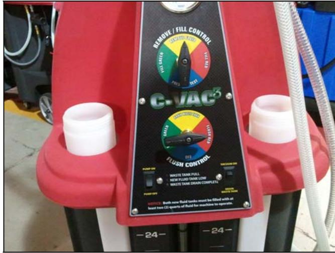
6. Turn on the “PUMP ON” and “VACUUM ON” switches and watch for fluid flow in the hoses.
